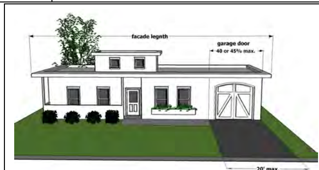
Figure 19.7.6-D: Maximum Driveway and Garage Door Width
