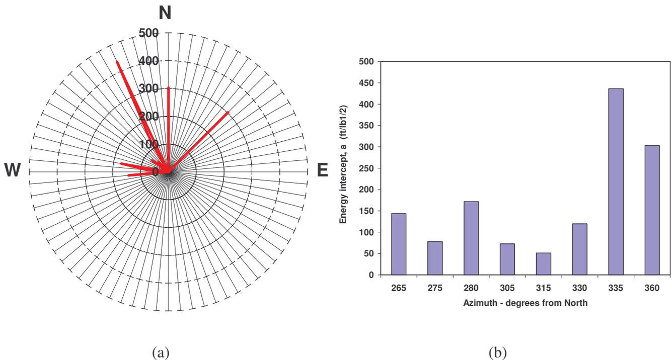
Figure 6 Variation of energy factor (y-intercept) values as a function of azimuth for (a) a circular distribution and (b) a conventional histogram
