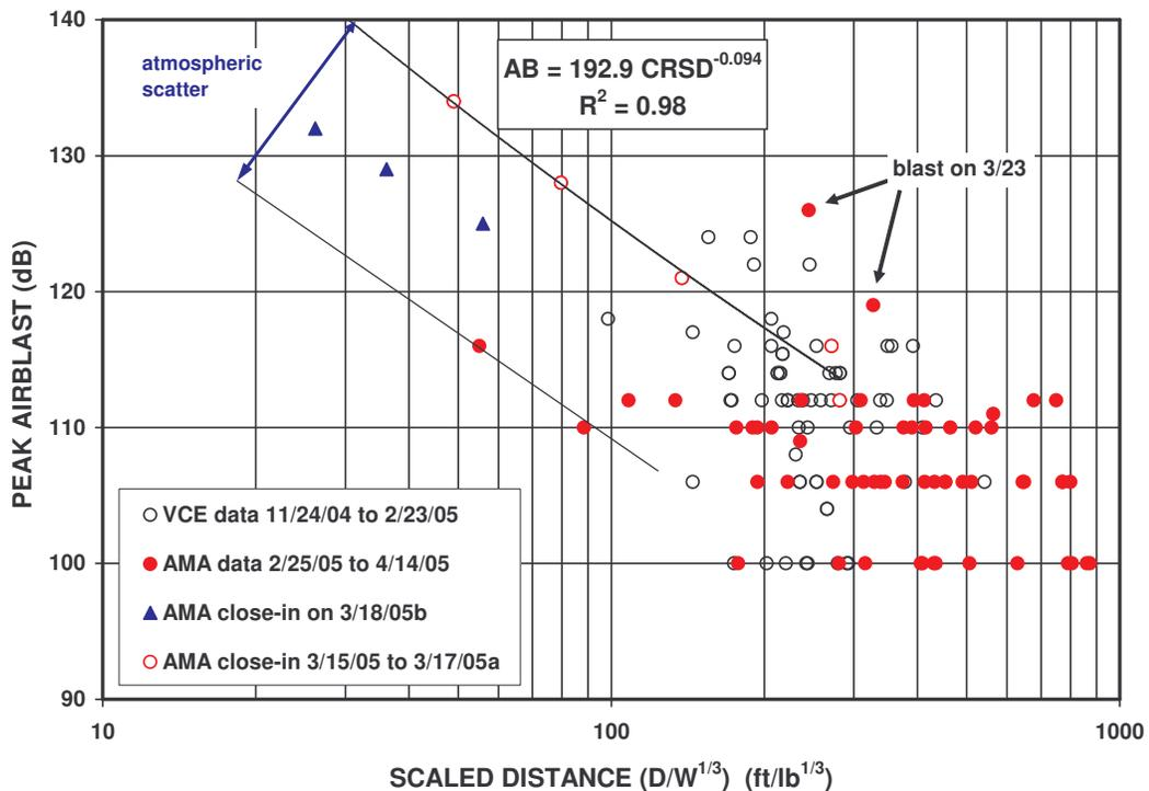
Figure 11 Peak airblast versus cube-root scaled distance
