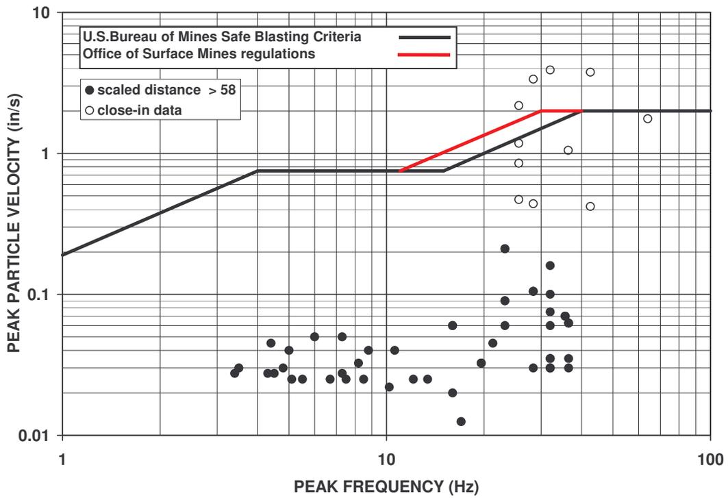
Figure 10 PPV versus frequency at the peak velocity for close-in adapt and far-field data (SD > 58 ft/lbs<sup>1/2</sup>)
