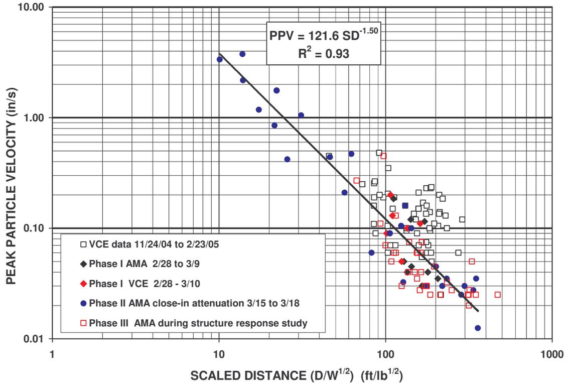
Figure 3 Peak particle velocity versus scaled distance
