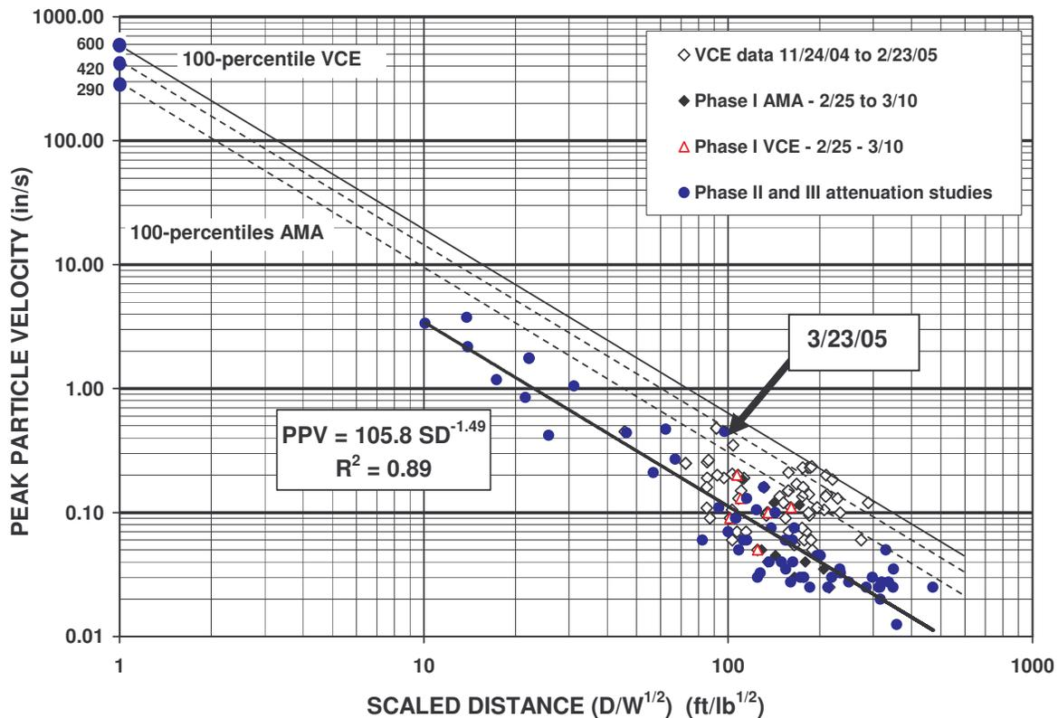
Figure 4 100-percentile attenuation lines for AMA data, Phases II and II combined and early data provided by VCE
