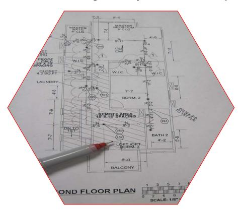
As a reminder, per NFPA 13, hydraulic reference points are required on the plans. hexagon reference Each point on the plan corresponds with reference point the hydraulic calculations.
