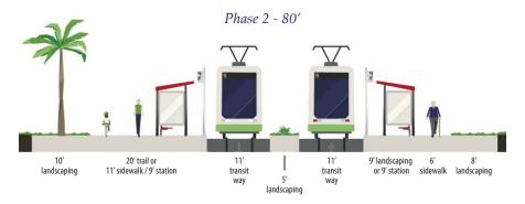
These cross sections conceptualize how desired elements and amenities can be incorporated into the major street network in West Henderson. The Master Streets and Highway Plan will need to be amended in order to adopt any of these alignments or cross sections, and changes and refinements are anticipated to be made. Please see the Master Streets and Highways Plan for currently adopted alignments.
