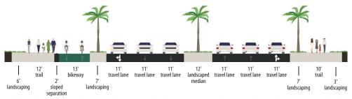
These cross sections conceptualize how desired elements and amenities can be incorporated into the major street network in West Henderson. The Master Streets and Highway Plan will need to be amended in order to adopt any of these alignments or cross sections, and changes and refinements are anticipated to be made. Please see the Master Streets and Highways Plan for currently adopted alignments.
