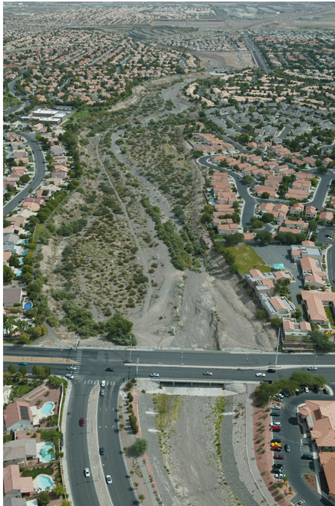
Aerial photos of Pittman Wash showing the contrast between concrete-lined channels and soft-surfaced channels.
